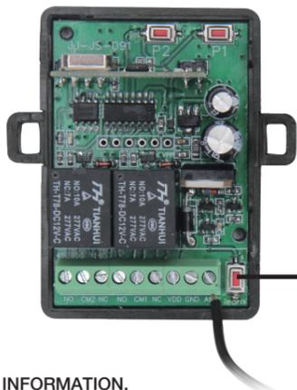
**LEARN BUTTON:** for pairing transmitter with receiver or to remove the transmitter.
